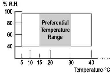
**Figure 1:** Humidity cure envelope for DOWSIL™ 895 Sealant.
