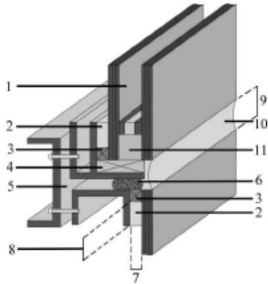
**Figure 4:** Design with supported insulating glass unit.
