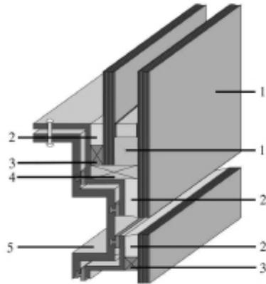
**Figure 5:** Design with stepped insulating glass unit.
